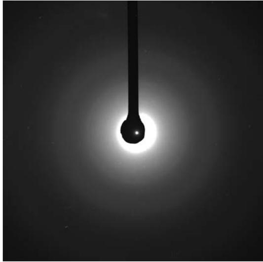
Fig. 4. Turbostratic structure of a particle from Figure 3. TEM, electron diffraction pattern
