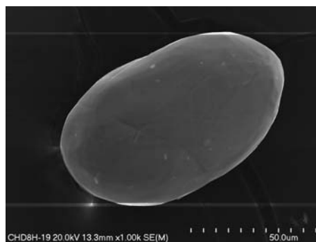
Phot. 5. SEM image of rounded zircon grain
