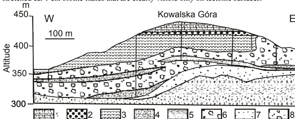
Fig. 10. Cross section of Kowalska Góra near Filipowice. Triassic: 1. dolomitic marls; 2. Bunter sandstone conglomerates. Lower Permian: 3. pyroclastic deposits; 4. epiclastic deposits, 5. Karniowice calcareous travertine; 6. Myślachowice conglomerates. Upper Carboniferous: 7. arkosic arenites. 8. sandstones intercalated with coals (based on Oberc et al. 1952 *vide* Parachoniak, Wieser 1985).
